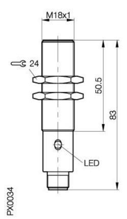
Inductive Sensors BES 516-366-S 4-C M18x1 x 83 normally-closed Sn=5mm shielded
